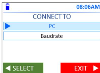
On the reader, go to **Settings > Connection > Cable > PC** to set the serial connection parameters.
