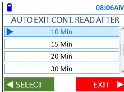
**Auto Mode** – This mode allows you to read one tag one at a time by pressing the **Read button** quickly or enters **Continuous Read** mode by pressing and holding the **Read button** for more than 1 second. When reading tags continuously, the reader beeps continuously and will issue 2 quick beeps if a tag is read and tag data is stored. Reading stops when the **Read button** is pressed again.
