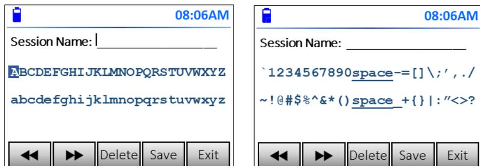
To delete a character, navigate to **Delete** using the ▲ ▼ ◀ ▶ **Keys** and press the **MENU/OK button** to delete a single character. To delete more characters, continue to press the **MENU/OK button** until all required characters have been deleted.
