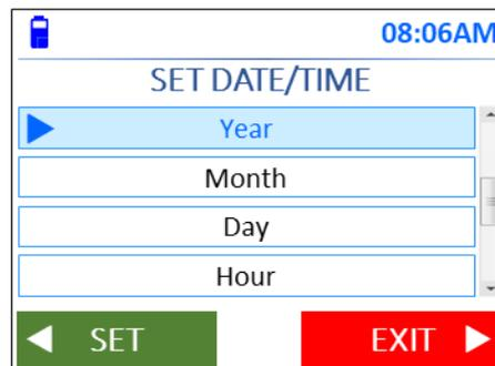
Use the ▲ / ▼ **keys** to navigate to each input field and press the ◀ **key** to select. Use the ▲ / ▼ **keys** to navigate to the appropriate values, then press **MENU/OK button** to save and exit.
