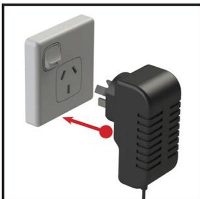
Plug the Battery Charger into the mains and power on. The Readers red LED indicates it is charging.
