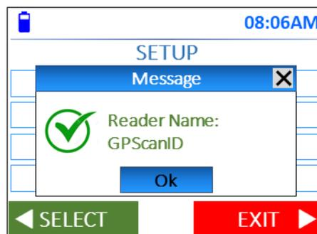
To exit the **Reader Name** set-up at any time, navigate to **Exit** using the ▲ ▼ ◀ ▶ **Keys** and press **MENU/OK button** to exit and return to the previous screen.
